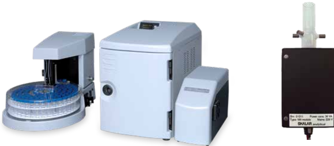
NO 2 and NO 3 Reactor
