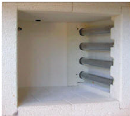
Heating Elements with Quartz Protective Tubing
